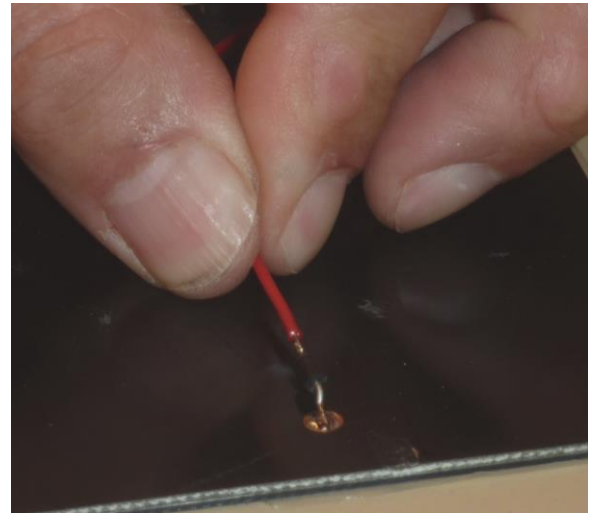
Solder the diode to the solar panel using the soldering iron and some solder wire
