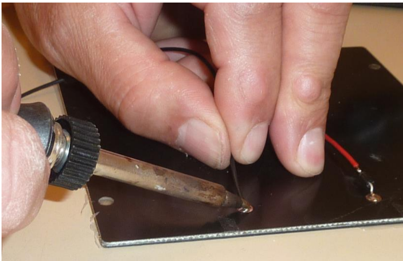
Solder the electrical wire to the solar panel
